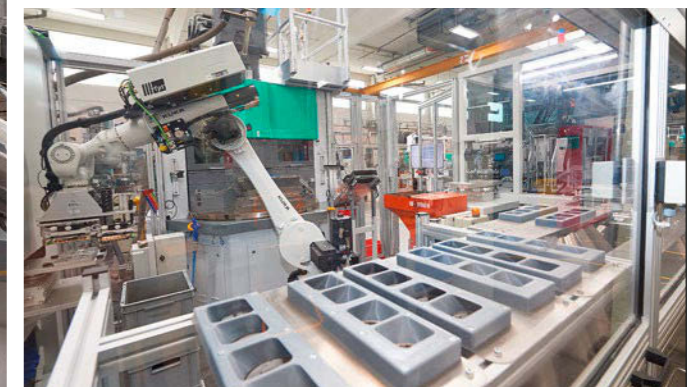
The precision pipes are available in different versions (large image left). The inserts are provided in the correct position by anyfeeders and a delta robot, inserted into the mould by the six-axis robotic system and overmoulded in a vertical ALLROUNDER with rotary table (images above right).
