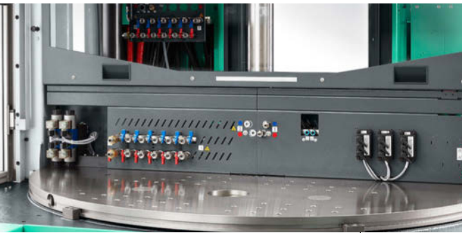
The tie-bar-free rotary table concept makes media connections easily accessible.
