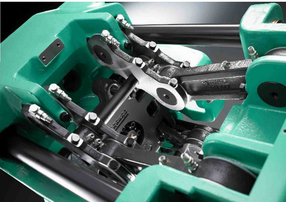
On the ALLROUNDER HIDRIVE (left) hydraulic valves and pressure accumulator are integrated in the machine base (centre left). The servo-electric toggle-type clamping unit (centre right) contributes to the energy efficiency of the ALLRDRIVE (below) and HIDRIVE machines.
