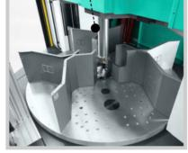
Tie-bar-free rotary tables of the V and T series: plenty of room for molds and media connections.
