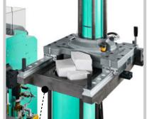
Material compatible: e.g. processing solid silicone (HTV) or moist polyester (BMC) with INJESTER tamping device.
