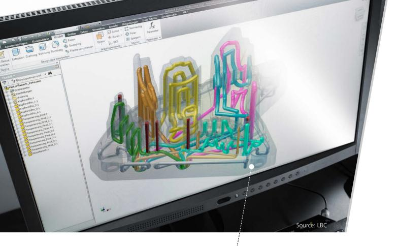
Near-contour mold temperature control reduces the cycle time and ensures high process control capability.
