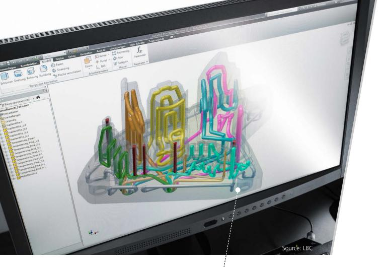
Near-contour mould temperature control reduces the cycle time and ensures high process control capability.
