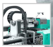
M position: second moving injection unit is mounted above the moving mounting platen.
