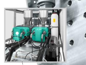
L position: second injection unit horizontal on the back of the machine.
