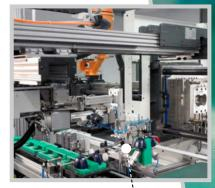
Fast and precise: the cavities of a multi-component mould are rotated by 120°. Individual turnkey solution: workpiece carrier circulation system connects two ALLROUNDERs.
