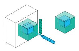
Sandwich structures in the component: with two specifically timed injection units.
