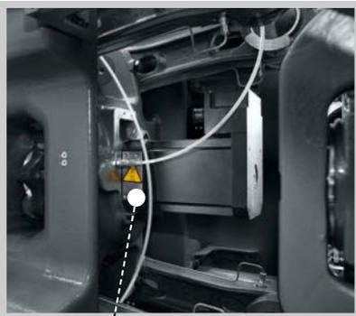
Servo-electric ejectors (optional): particularly precise dropping of molded parts for even shorter cycle times.
