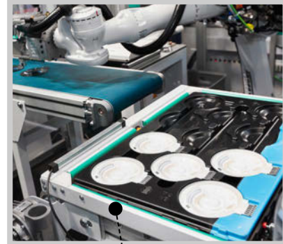
Film insert molding: excellent reproducibility with servo-electric drives.
