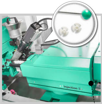
Micro injection molding extremely small shot weights thanks to the size 5 micro-injection unit.
