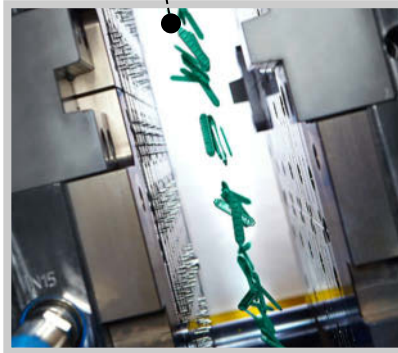
Film insert moulding: excellent reproducibility with servo-electric drives.
