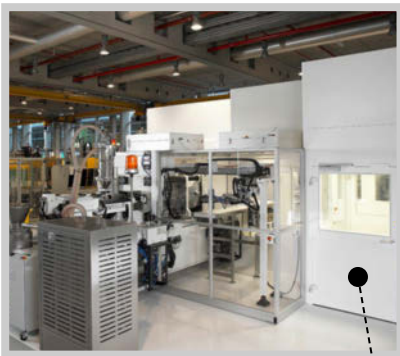
Inserts for blood flow diverters: safe overmoulding in docked-on production cell.
