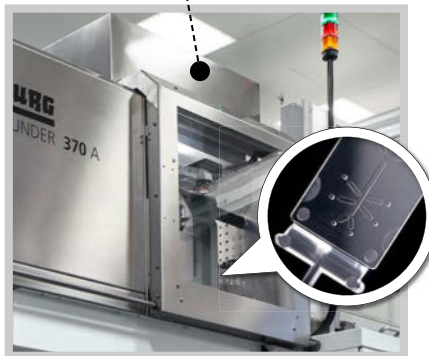
Particle-free in-mould lamination of display foils: individual turnkey solution from a single source.
