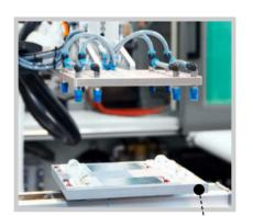
Control of complex processes: injection compression molding of high-quality optical lenses.
