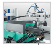
Process reliability: the cylinder module with liquid temperature control helps prevent premature cross-linking.
