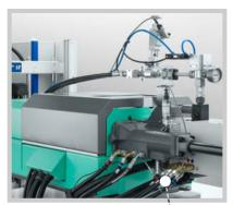
Process-reliable: the cylinder module with liquid temperature control helps prevent premature cross-linking.
