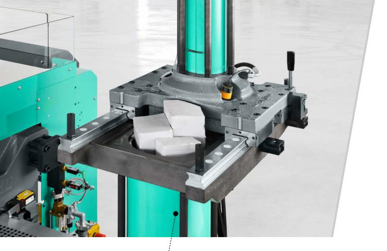
Material-specific: feed via INJESTER tamping device.
