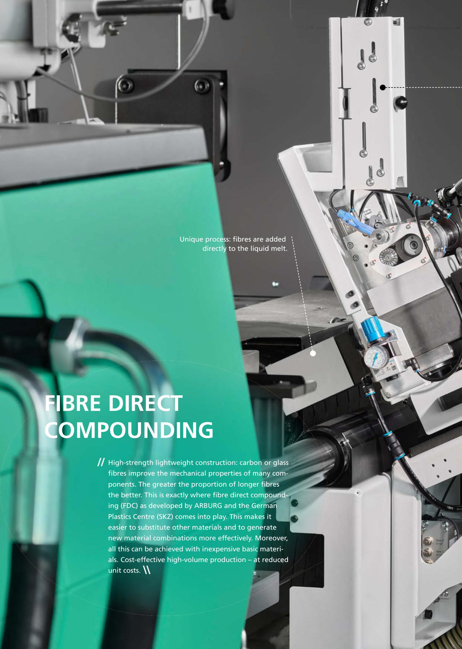
Unique process: fibres are added directly to the liquid melt.
