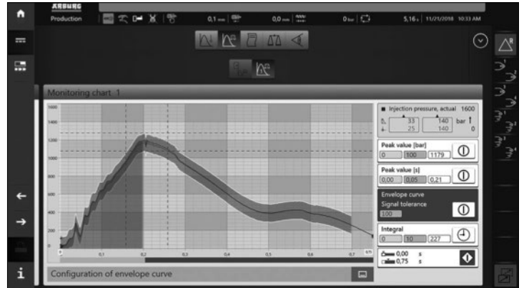
Detailed monitoring: use the „Monitoring via actual-value graphic“ function to detect process deviations early.
