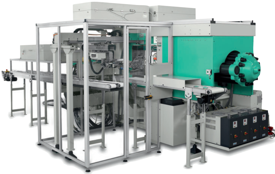
Fig. 5. Flowboxes are integrated in the production cell for ophthalmic lenses
