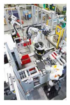
Fig. 6. Synchronized trio: a six-axis robot delivers metal inserts with positional accuracy, the second robot takes the inserts and contacts and places them in the mold, while the third robot is responsible for the inspection of the finished parts by camera
