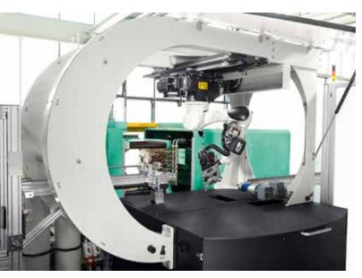
One of the advantages of the mobile cell is the larger operating zone available, as the small six-axis robotic system moves along a seventh linear axis (figures: Arburg)
