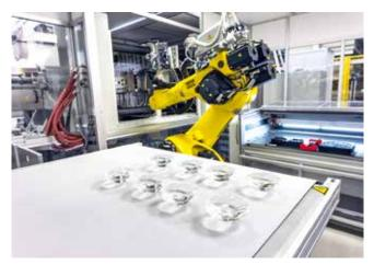
**Fig. 8.** While the thick lenses cool in the mold, the six-axis robot transfers more products for laser processing (rear right in the figure) (figure: Erco, Dirk Vogel)
