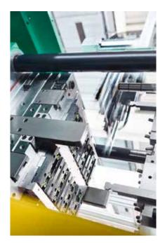
Fig. 4. For highspeed applications, a linear robotic system with a fastaction mold-entry axis may be a better option than a specially designed automation solution
