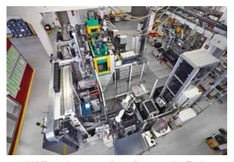
**Fig. 7.** H&B Electronic uses a complex turnkey system. Handling is performed by three six-axis robots, plus two linear robotic systems traversing on a cross head. All communication is handled by the central machine control system
