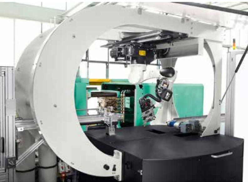
One of the advantages of the mobile cell is the larger operating zone available, as the small six-axis robotic system moves along a seventh linear axis (figures: Arburg)
