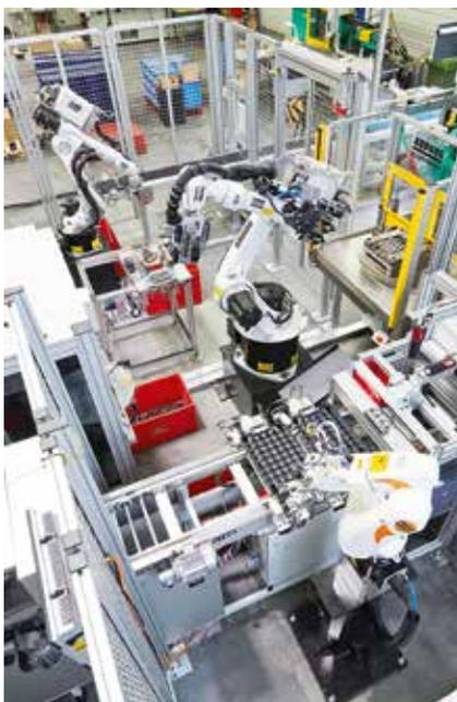
**Fig. 6.** Synchronized trio: a six-axis robot delivers metal inserts with positional accuracy, the second robot takes the inserts and contacts and places them in the mold, while the third robot is responsible for the inspection of the finished parts by camera
