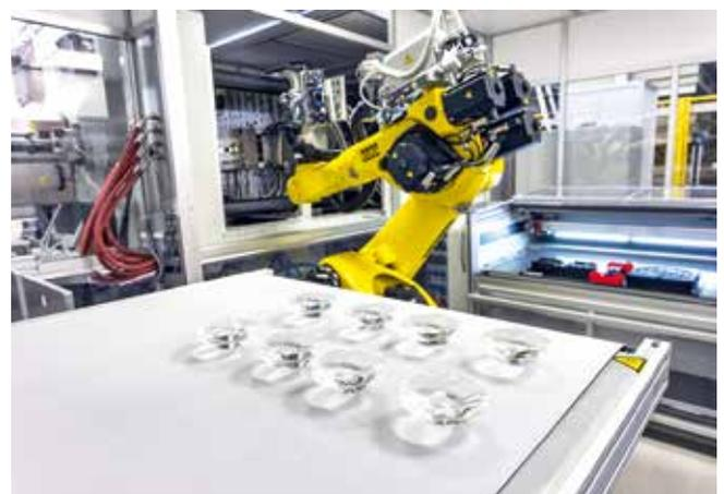
**Fig. 8.** While the thick lenses cool in the mold, the six-axis robot transfers more products for laser processing (rear right in the figure)
