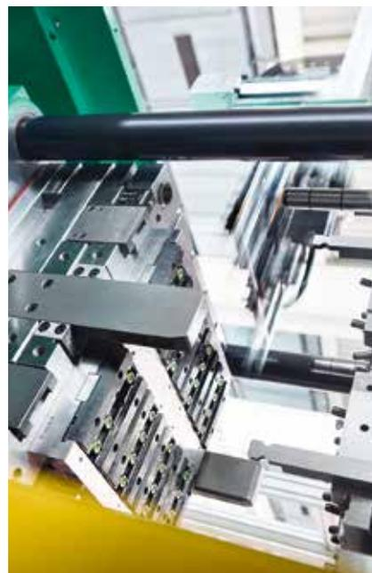
**Fig. 4.** For high-speed applications, a linear robotic system with a fast-action mold-entry axis may be a better option than a specially designed automation solution
