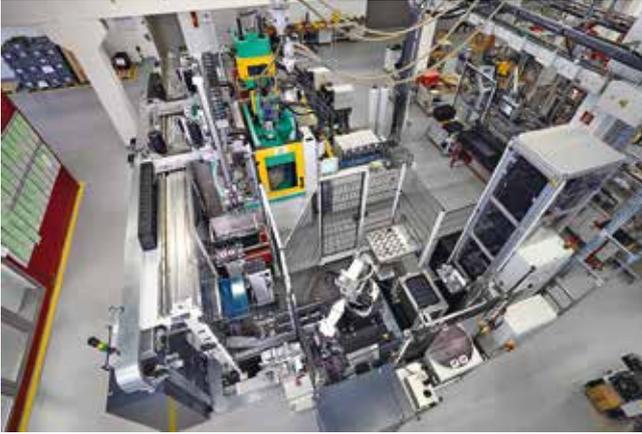
**Fig. 7.** H&B Electronic uses a complex turnkey system. Handling is performed by three six-axis robots, plus two linear robotic systems traversing on a cross head. All communication is handled by the central machine control system
