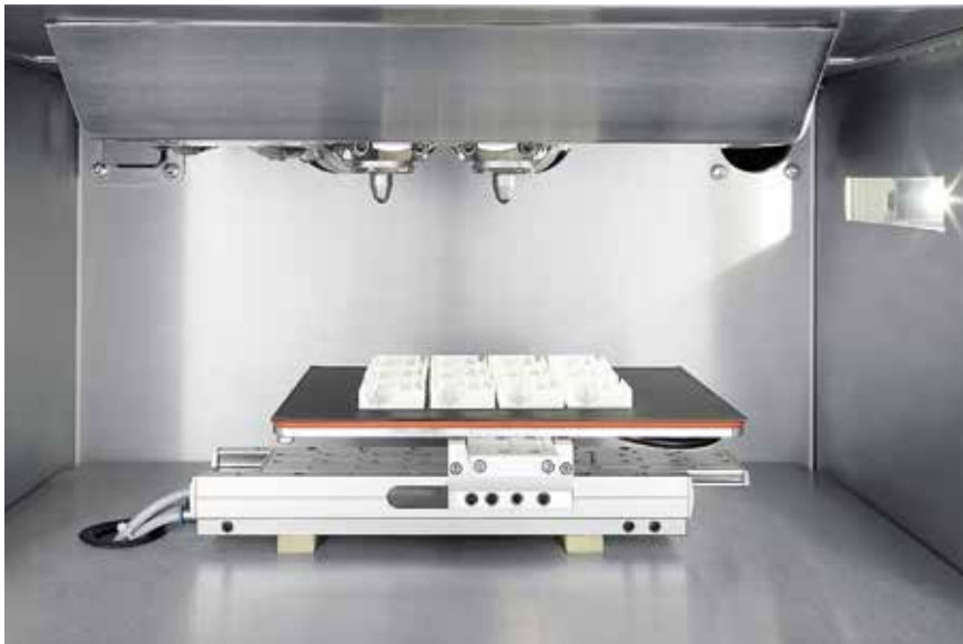
Fig. 2. At the Arburg Technology Days 2014, a Freeformer produced twelve connector housings made from ABS as spare parts for Allrounder injection molding machines
