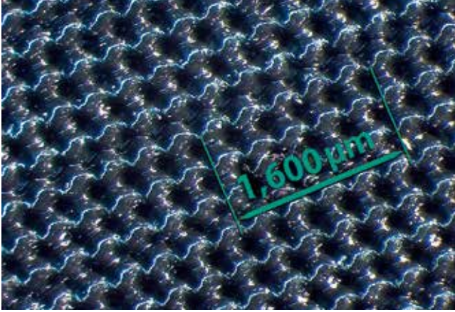
Fig. 3. The macro image (48 x magnification) of a surface created using the Freeformer shows the homogeneous, dense, layered structure
