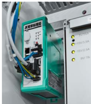
Flexible machine – Basic connectivity with OPC UA
