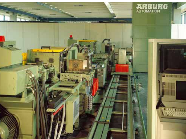
A sight from the past: ARBURG automation as a showpiece of the CMD era with several ALLROUNDERS, in fully-automated operation, controlled via a host computer.
