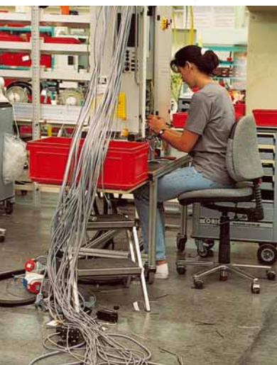
Control cabinet assembly
