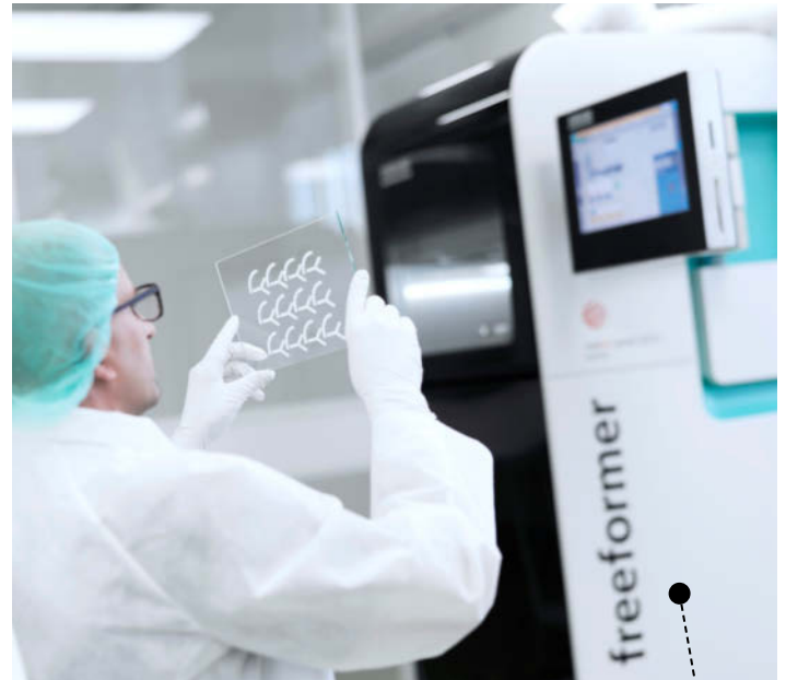
Additive manufacturing of implants with the freeformer
