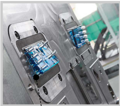
"Ready-to-use" lab-on-a-chip: complex assembly injection moulding using two components.
